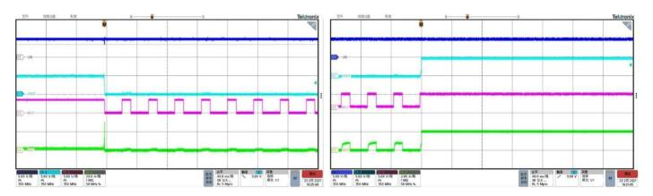
output short circuit with 2.5 $\Omega$  load
